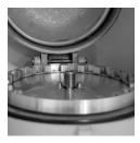
This test determines the effects of types of structural and/or mechanical weaknesses that may not have been detected in vibration tests. Uses vary from determining the mechanical limits of the package of the device, internal metallization, die or substrate attachment and other elements of the device
